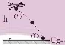
$$\Rightarrow h = \frac{v_f^2 - v_i^2}{2g} \xrightarrow{v_f = 25 \frac{m}{s}, v_i = 54 \frac{km}{h} = 15 \frac{m}{s}}$$
